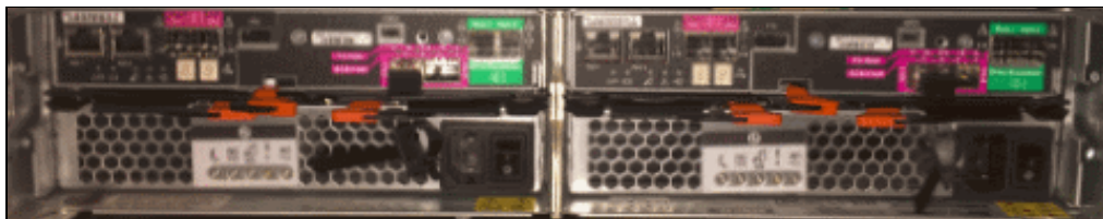
Figure 7-8 TS7760 Cache Controller 3956-CSA (rear view)
